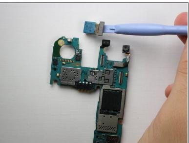
Use a plastic opening tool or spudger to pry off the rear-facing camera from the motherboard.
