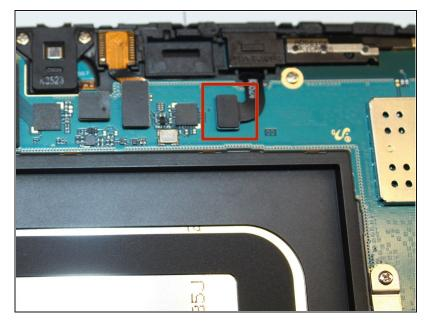
• With a plastic remover tool, gently unseat the connection of the proximity sensor to the motherboard.
