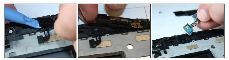
• Gently wedge the plastic remover tool and pry antenna loose, and lift it from the proximity sensor. The Sensor can then simply lifted from the device.
