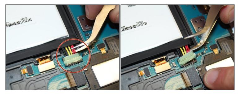
• To remove the battery you must use something small, such as tweezers, to disconnect the battery from its port.
