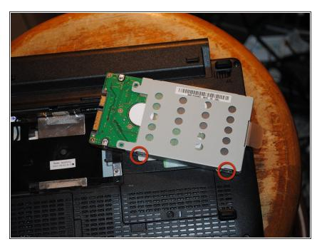
Remove hard drive from computer and loosen 4 screws that hold it into it's metal housing.
