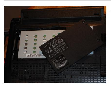
Next, loosen both screws and remove plastic door.
