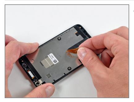
• Peel the front panel ribbon cable off the adhesive securing it to the metal underside of the inner case.
