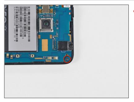
Remove the single Phillips screw securing the motherboard to the inner case near the headphone jack.
