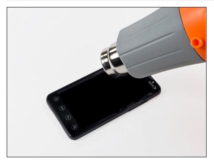
Use a heat gun to soften the adhesive along the left side of the front glass panel.
