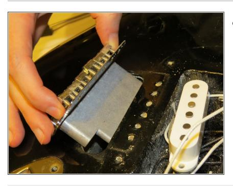
With all six screws removed, lift up on the bridge to remove it from the body.
