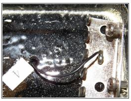
Be aware that the ground wire for the electronics of the guitar is routed through the body and soldered to the spring retainer.
