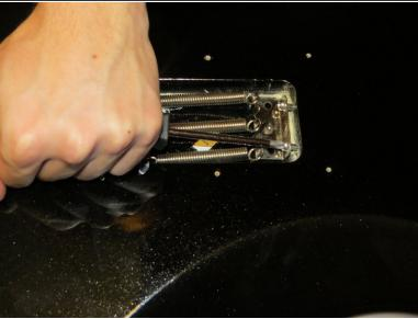
On the back of the guitar, remove the plate covering the spring cavity. In the spring cavity, reduce the tension on the bridge springs by first loosening the retainer screws a bit.
