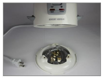
Carefully lift up the device, either by allowing the hotplate portion to fall out while it is close to the ground, or by catching the hotplate portion as it slides out.
