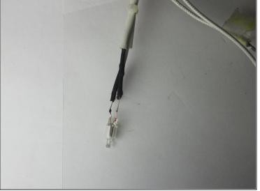
Using a sautering iron, carefully sauter both wire ends of the new light bulb to the device's wires.
