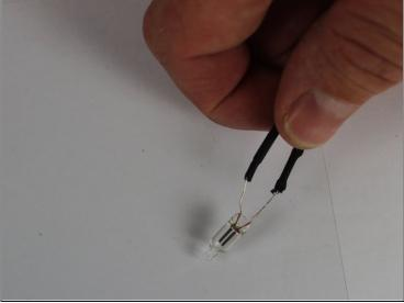
Using a pair of needlenose pliers or wire strippers, cut the rubber covering on each wire about
