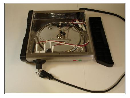
Plastic sides should be easily removed after all screws are taken out.
