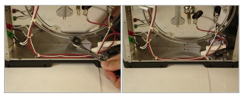
Using a #1 Phillips screwdriver bit or a ratchet wrench with a Phillips screwdriver bit to remove screws located on the interior frame.
