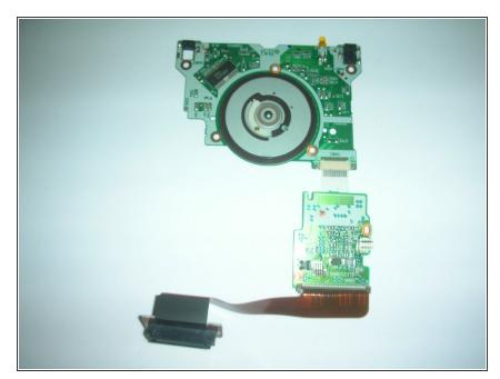
Here is an isolated image of the core hardware of the floppy drive.
