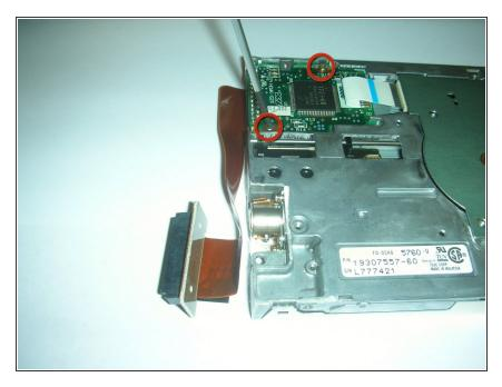
Remove the two screws holding part of the floppy processing unit.
