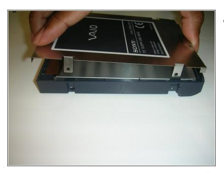
Remove the floppy drive core from its casing.
