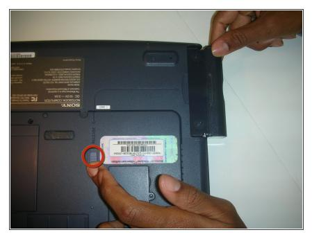
Turn the device over so that its underside is facing up. Then, slide the blue floppy drive release button down and pull the floppy drive out of the laptop.
