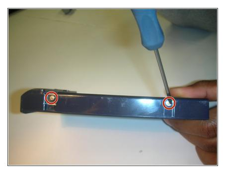
There are two screws on each side of the floppy drive (four screws total). Remove these screws.
