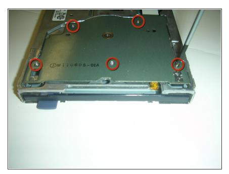
Unscrew the five screws from the back of the optical drive.
