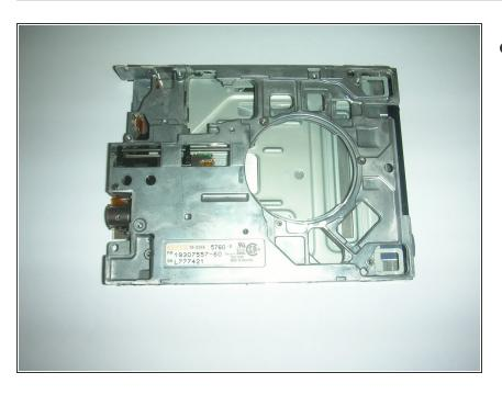
Here is an isolated image of the floppy drive casing unit.
