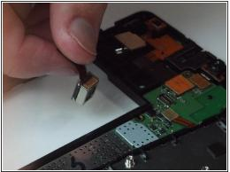
Gently pull the motherboard connector upward to remove the rear camera component.
