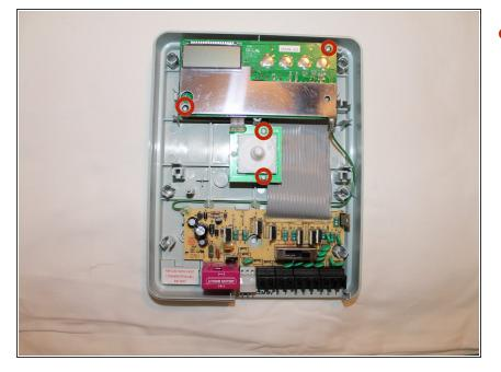
• Use a Phillips #0 screwdriver to remove the four 6mm screws.
