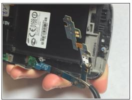
With your tweezers remove the bottom circuit from the screen.
