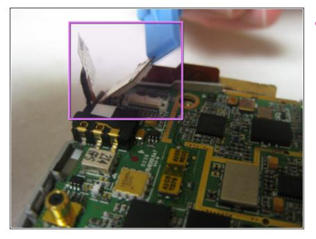
Remove the clip from the logic board.
