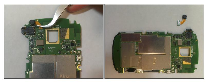
(i) The front facing camera is attached to the back of the motherboard by a single cable ribbon.
