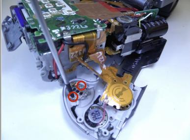
Unscrew the two Phillips #00 1.6x3mm screws that hold in the trigger button.
