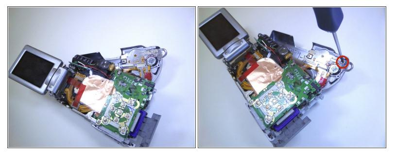
Unscrew the Phillips #00 1.6x3mm screw located on the top panel.
