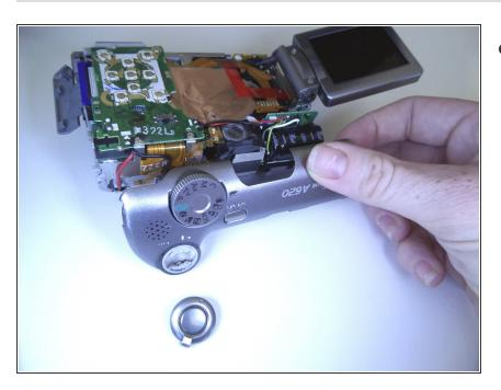
The trigger button will fall off once the screws have been removed.
