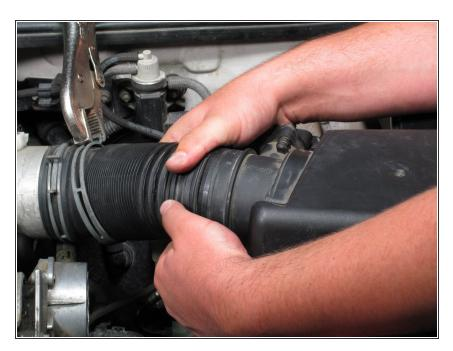
Pull the intake tube off of the air filter cover.
