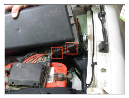
Lift the air filter cover up, starting from the back end, making sure to release them from the hinges on the front end.
