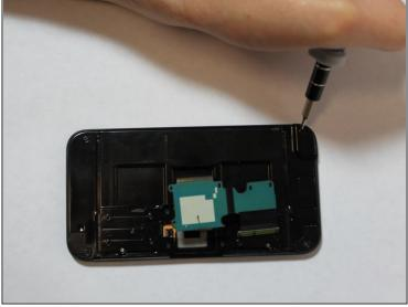
• Remove the four corner screws using the #00 screwdriver.
