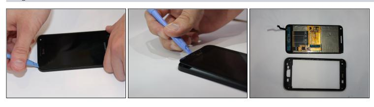
• Using the plastic opening tool to pry around the edges, release the touch screen from the screen frame.
