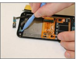
• Use the plastic opening tool to release the main jaw connector, front speaker and camera.
