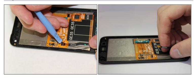
By using the plastic opening tool you can release the keypad flex cable from the jaw connecter clamp.
