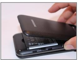
Remove back cover using fingernail or plastic opening tool. The cover pulls up and off.
