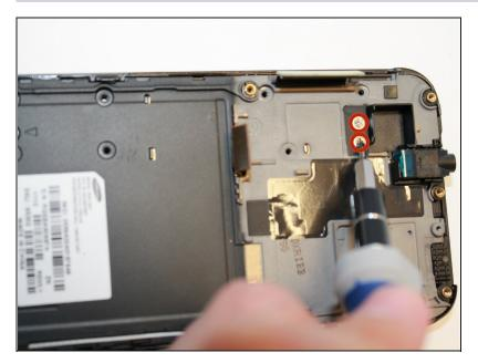
• Remove screws with the #00 screwdriver.
