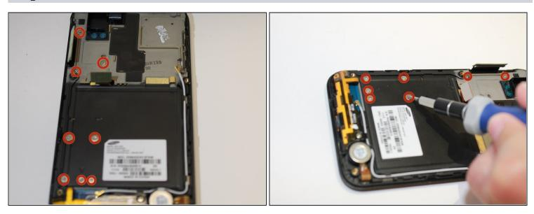
Remove the eight screws with the #00 screwdriver.
