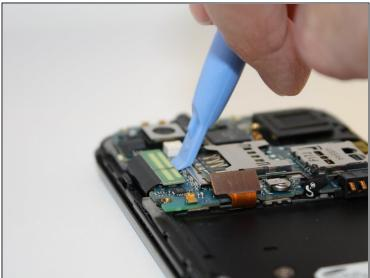
• Use the plastic opening tool to detach the two tabs connecting the motherboard to the base of the phone.
