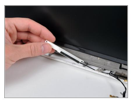
Remove the center antenna from the display assembly.
