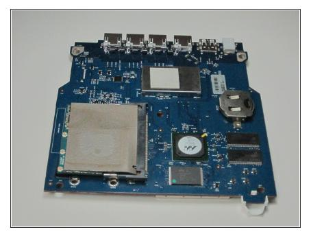
Carefully pull the metal case away from the logic board.
