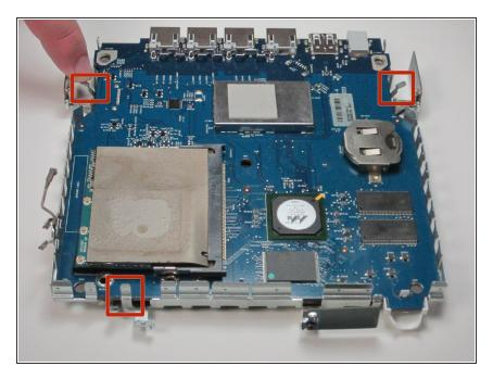
Carefully push back the three metal tabs with your fingers on the sides of metal case.
