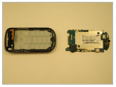
If intending to reuse the logic board, be sure to place it in a space that minimizes contact with dust and dirt.
