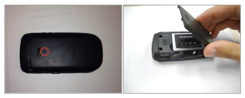
• Detach the battery cover by sliding the cover down toward the bottom of the phone.
