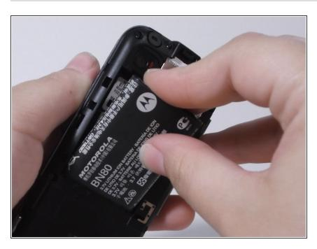
Locate battery and use your index finger to grasp the upper left side of the battery and pull back to remove. Set battery aside.
