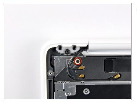
Remove the single 3 mm Phillips screw securing the AirPort/Bluetooth antenna ground strap to the rear speaker.
