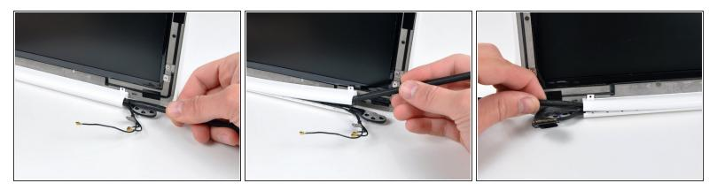
Insert the flat end of a spudger into the open end of the clutch cover and pry up to release it from the rear display bezel.
