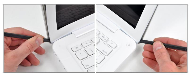
Carefully pry up the front display bezel where it is stuck to the display assembly near the clutch hinges.
