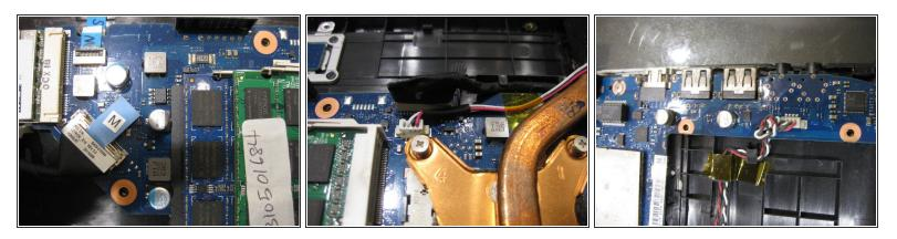
removing the Main PCB means detaching the cable marked M, W the big fat black cable at the top and the white connector at the right usb side.
