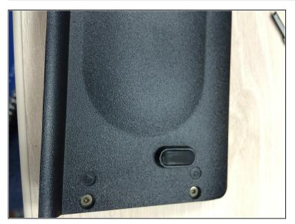
Remove the two screws marked "4" from the hard drive cover
