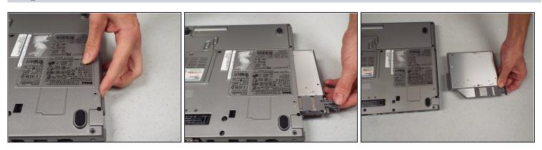
• Remove the CD/DVD drive by pushing on the button under the drive.
