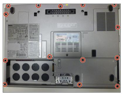
• Remove the 14 Phillips screws from the bottom of the laptop.
