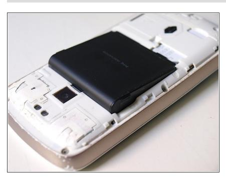
Take out the battery using the two tabs at the upper right and upper left corner of the battery.
