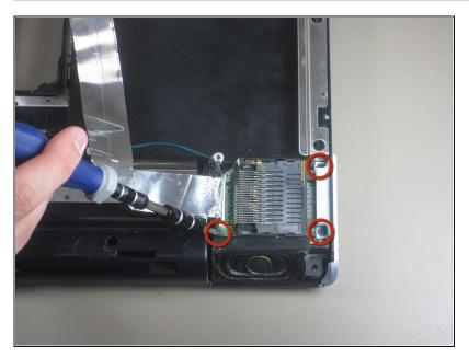
Remove the 3 screws connecting the spearker.
