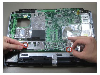
• Disconnect the speaker cables from the motherboard.
