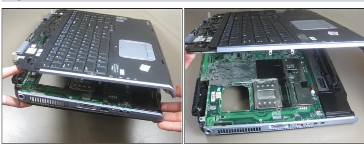
$\triangle$  Do not remove the keyboard yet! There are still wires connecting the two components.
