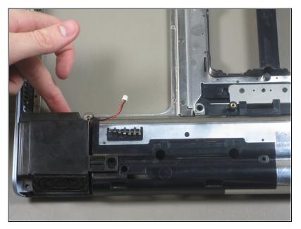
• To remove the second speaker simply lift it up and out.
