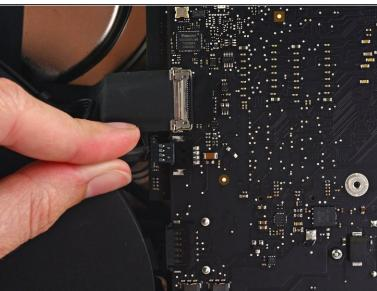
Gently pull the fan cable connector straight away from its socket on the logic board.
