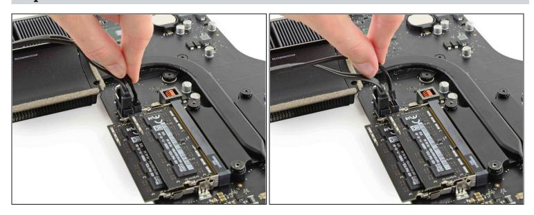
Grasp the hard drive power connector and gently pull it out of its socket on the logic board.
