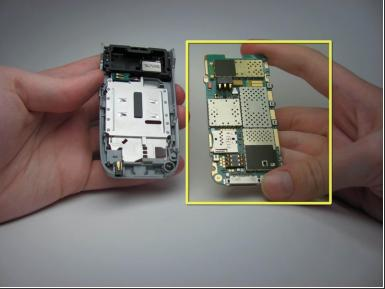
Remove the logic board from the back cover of the phone.
