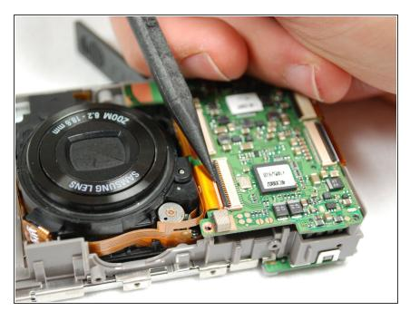
Use spudger to remove ribbon connecting the circuit board from lens.
