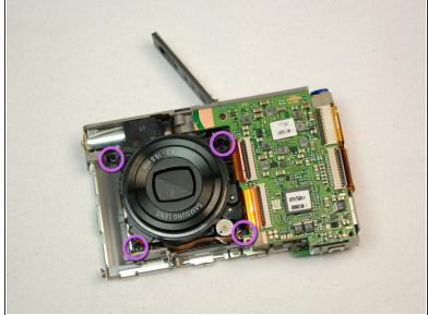
Remove four screws around lens.
