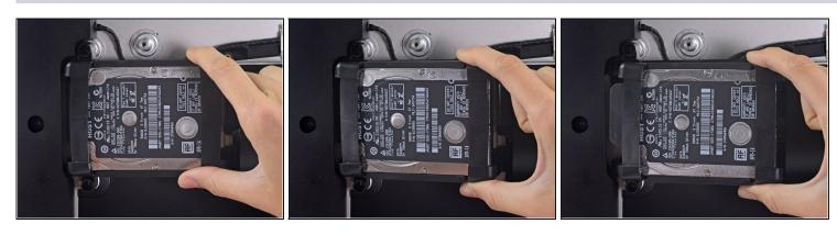
• Lift the hard drive from the edge nearest the logic board and pull it slightly out of its recess.
