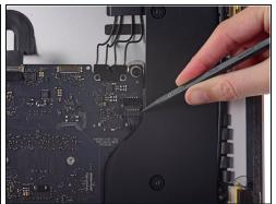
• Use the tip of a spudger to push on either side of the right speaker cable connector to walk it out of its socket on the logic board.
