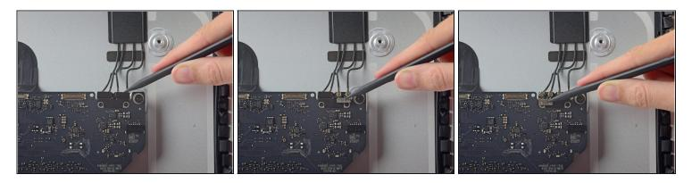
(i) If necessary, use the tip of a spudger to peel back the tabs covering the antenna connectors.
