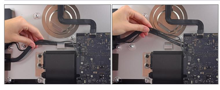
• In a similar fashion as the previous step, de-route the combo SATA data/power cable up out of the retaining clip.
