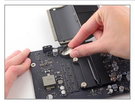
Lift and remove the PRAM battery off the logic board.
