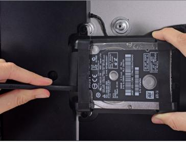
• Use a spudger to disconnect the single SATA power and data combo cable by gently prying its large plastic connector away from the hard drive.
