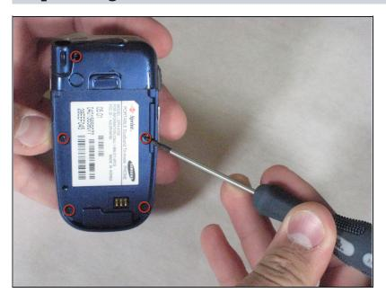
• Remove the five screws as shown.
