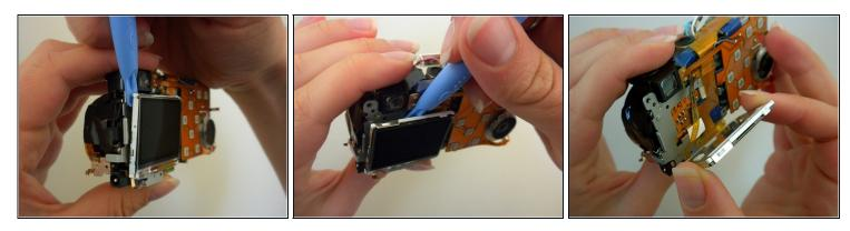
• Pry off the LCD screen from the top using an opening tool.
