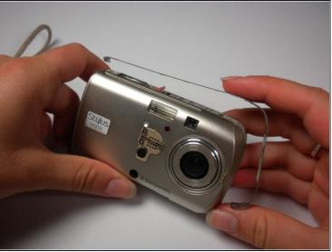
Use the spudger to peel off the outer metal band, starting from the bottom of the camera.
