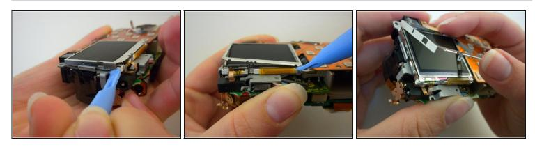
• Remove the metal frame from the LCD screen using an opening tool.
