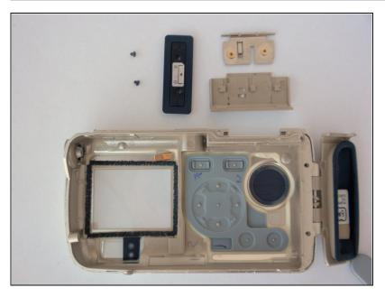
This is what the battery cover and back case look like completely disassembled.
