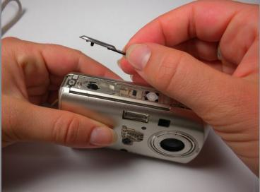
The shutter button can now be removed. It is not connected to the camera and can be lifted off.
