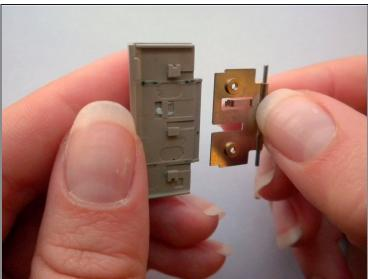
Slide the metal piece off of the battery cover.
