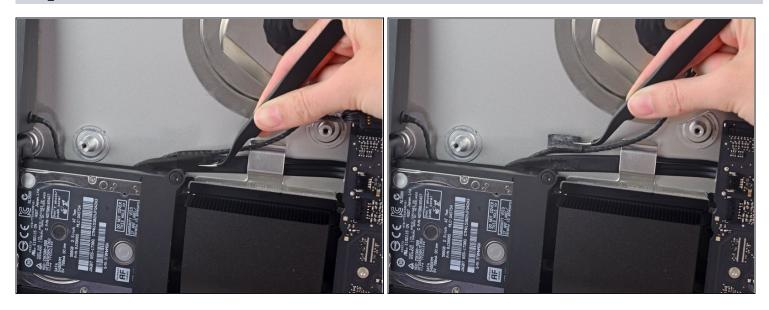
• Use a pair of tweezers to gently peel the tape securing the left speaker cable to the SATA data/power cable.
