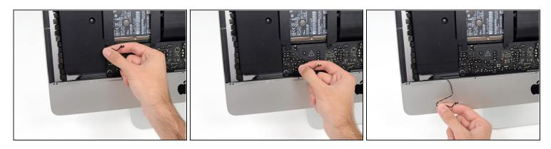
• Carefully de-route the power button cable from its groove in the left speaker.
