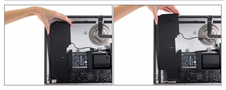
• Lift the left speaker straight up and remove it from the iMac.
