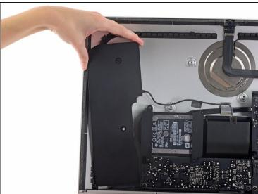
Lift the left speaker straight up, until the power button cable is exposed (about 0.5").
