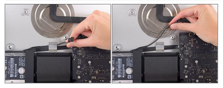
• Lift the left speaker cable upwards to de-route it from the clip holding it to the rear case.
