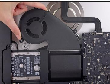
• Gently lift the fan up and remove it from the iMac.
