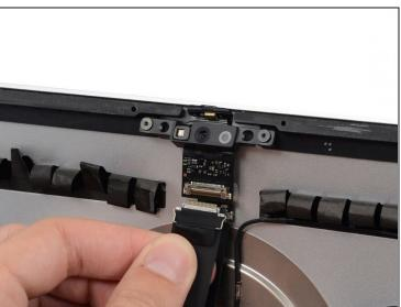
Gently pull the iSight camera cable straight down and out of its socket on the camera board.
