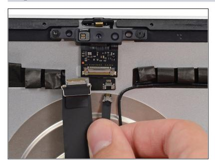
Pull the microphone cable connector straight down out of its socket on the camera board.
