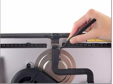
• Use a pair of tweezers to grasp and flip the metal retaining bracket downwards to free the iSight camera cable connector.
