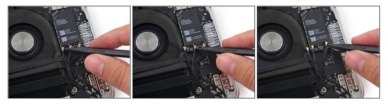
• Insert the tip of a spudger under each of the antenna cables near their connectors and pry up to disconnect them from the AirPort board.
