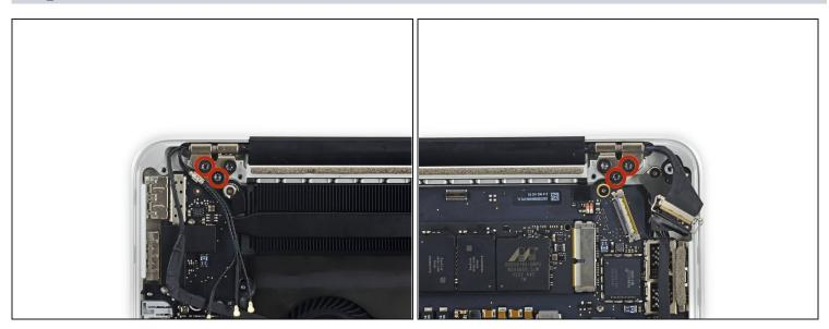
Remove the four outer 5.3 mm T8 Torx screws (two on each side) securing the display to the upper case.
