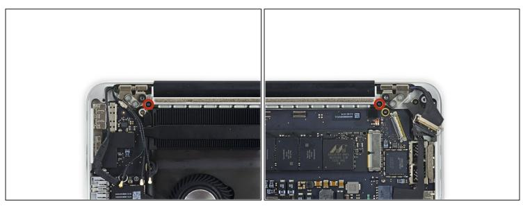
Remove the two 4.2 mm T5 Torx screws securing the aluminum hinge brackets (one on each side of the Macbook).
