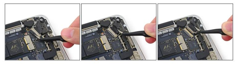
• Grab the black plastic tab to flip the display cable connector open and pull it straight out of its socket on the logic board.
