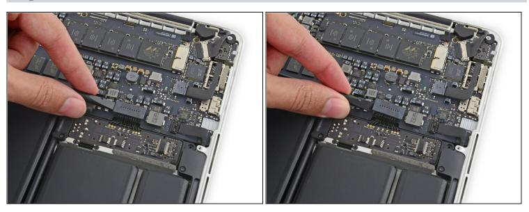
• Use the flat end of a spudger to lift the battery connector straight up out of its socket on the logic board.
