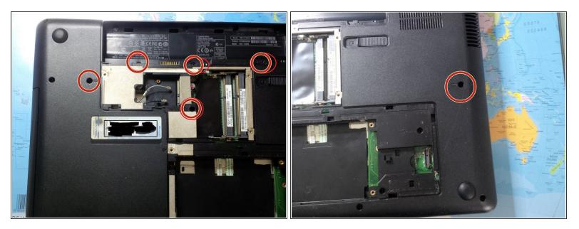
Remove the 6 keyboard screws.
