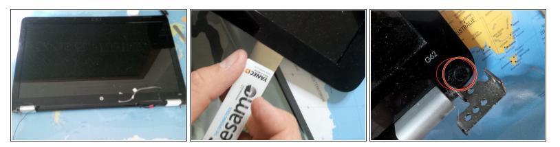
• if you have to remove the LCD screen connector you have to remove the case arround the screen. same thing if you have a broken screen..
