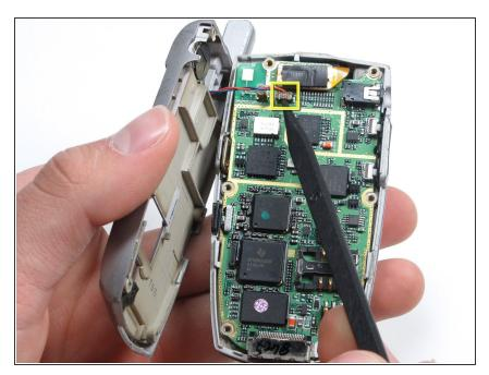
Use a spudger to disconnect antenna wire.
