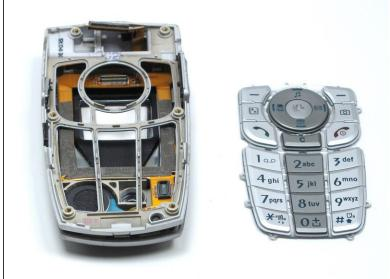
Using a spudger, lift the keypad off of the tabs.
