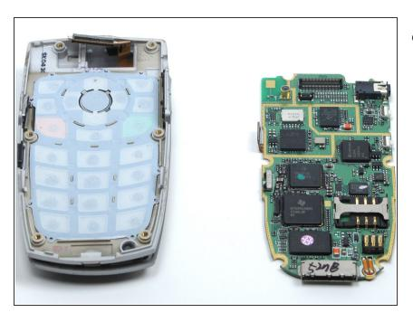
Once the ribbon is detached, remove the logic board and replace if necessary.
