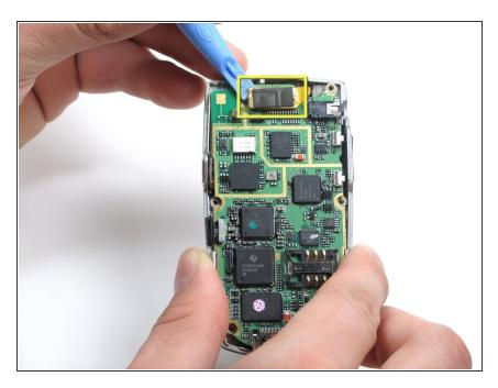
Use the IPod opening tool to disconnect the main ribbon.
