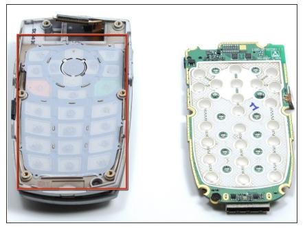
The back of the keypad is shown here, next to the logic board (the logic board is turned over to expose the buttons).
