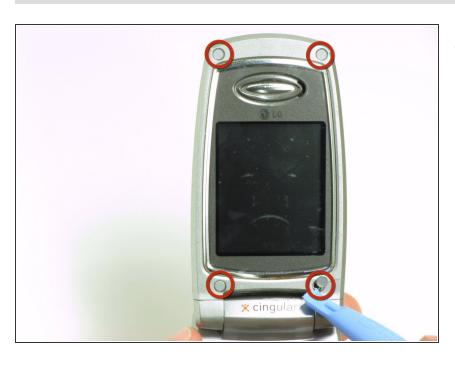
Remove all four screw covers by using an IPod opening tool. They should come off relatively easy.
