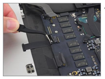
Pull the trackpad ribbon cable straight out of its socket on the logic board.
