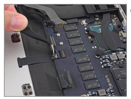
i If necessary, peel back any tape covering the trackpad cable connector.
