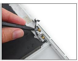
• Insert the tip of a spudger under the connector end of the microphone ribbon cable and lift to peel that section up from the upper case.
