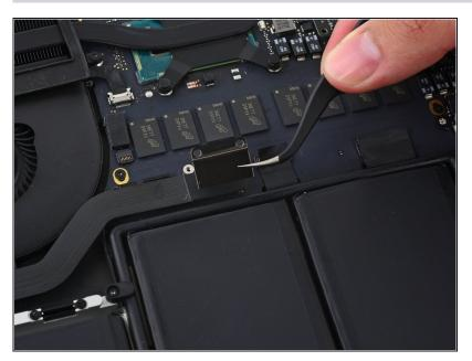
Grasp the I/O board cable bracket with a pair of tweezers and remove it from the MacBook.
