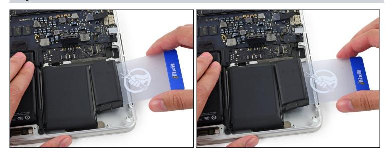
• Use the plastic card to pry the right-most battery cell up from the rear case.
