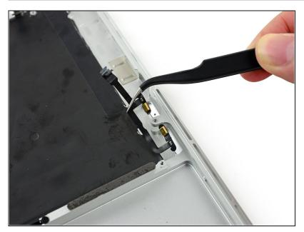
• Remove the microphone cable from the upper case.
