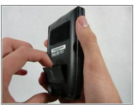
Turn the device over so it is face down and remove the stylus, and battery cover.
