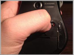
Power off the mouse. The power switch is located on the bottom of the mouse above the battery.
