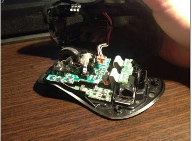
Carefully pry off the top of the mouse. This will remove the housing from the circuit board.
