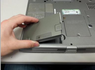
Pull the tab to release the battery
