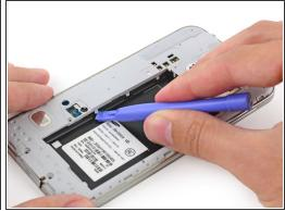
Gently run a plastic opening tool down along the left inner side of the interior frame to separate the three white plastic clips.
