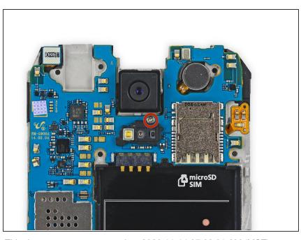
Remove the single 3.0 mm Phillips #000 screw securing the motherboard to the midframe.
