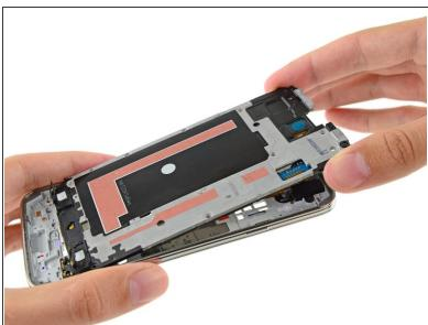
• Carefully remove the interior midframe/motherboard assembly from the white inner midframe.
