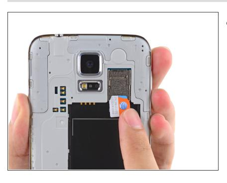
Repeat the above procedure to remove the SIM card.
