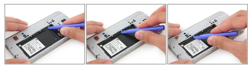
• Gently run a plastic opening tool down along the left inner side of the interior frame to separate the three white plastic clips.
