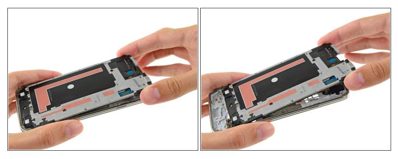
• Carefully remove the interior midframe/motherboard assembly from the white inner midframe.
