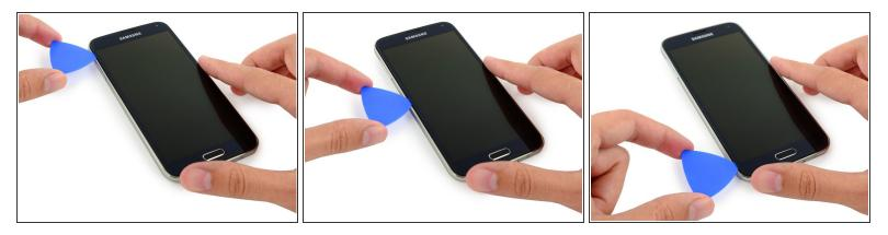
• Slide the opening pick down along the left half of the phone stopping at the lower left corner.
