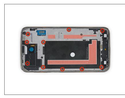
Remove the ten 3.4 mm Phillips #000 screws from the display side of the midframe.
