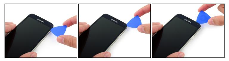
Carefully slide the pick around the corner, stopping before the speaker grille at the top of the phone.
