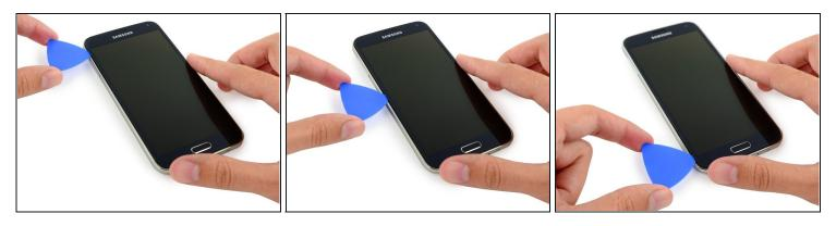
• Slide the opening pick down along the left half of the phone stopping at the lower left corner.
