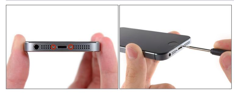
Remove the two 3.9 mm Pentalobe screws next to the Lightning connector.
