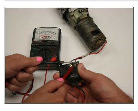
Use a multimeter set above 18V DC to check electrical connections where wires meet drill, switch, or battery terminal.
